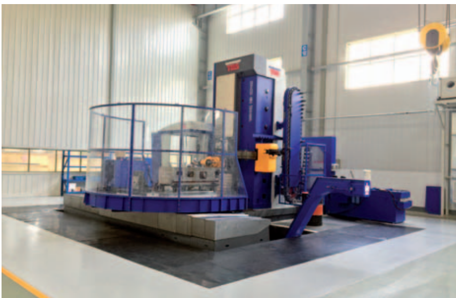
WHQ 13 CNC Hiecise Heavy – duty Machines Co., Ltd. – China X = 3 500 mm (137.7952 inch) Y = 2 500 mm (98.4251 inch) Z = 1 600 mm (62.9921 inch) ATC = 60 Table clamping surface = 1 800 x 2 200 mm (12 tonnes) 70.8661 x 86.6141 (13.2 tons)
