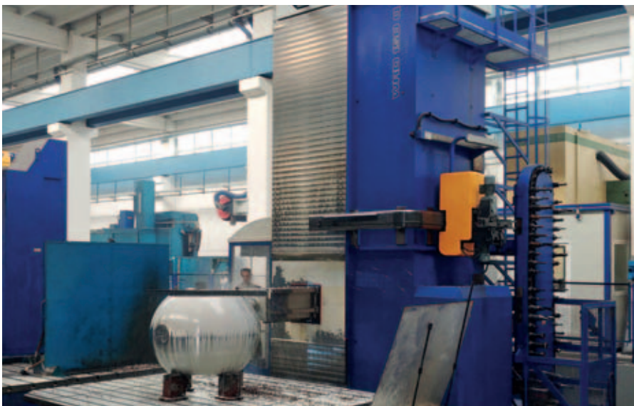
WRD 150 Q Tecnoweld Italia srl – Italy X = 11 000 mm (433.0708 inch) Y = 4 500 mm (177.1653 inch) ATC = 60 Table clamping surface = 3 000 x 3 500 mm (50 tonnes) 118.1102 x 137.7952 inch (55.1 tons)
