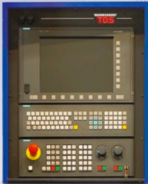
CONTROL PANEL OF SINUMERIK 840 D CONTROL SYSTEM
